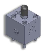
The Covers with Stroke limiter model H9-LC\*STS\* are designed to hold Hydronine make Cartridge valves in cavities machined as per ISO 7368, and control opening and closing of the cartridge valve by electrical signal. Effective closing pressure is the pressure from either port 'X' or 'Z1', which ever is higher.
